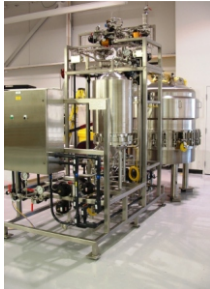
Viral Removal Skid
